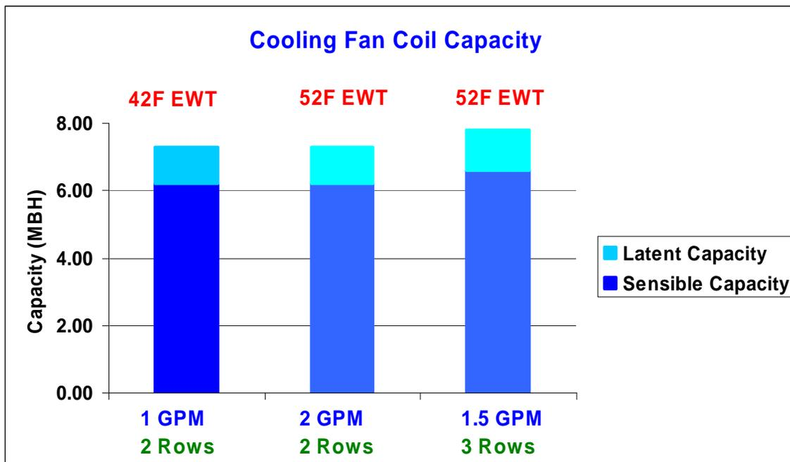
Figure 1 – Cooling Coil Capacity
