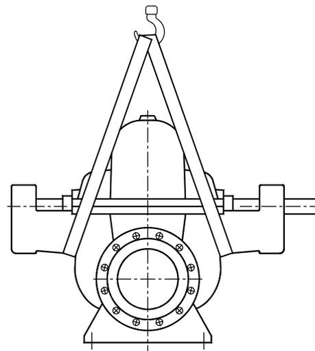
Figure 1: Attaching a Sling to the Pumpset
