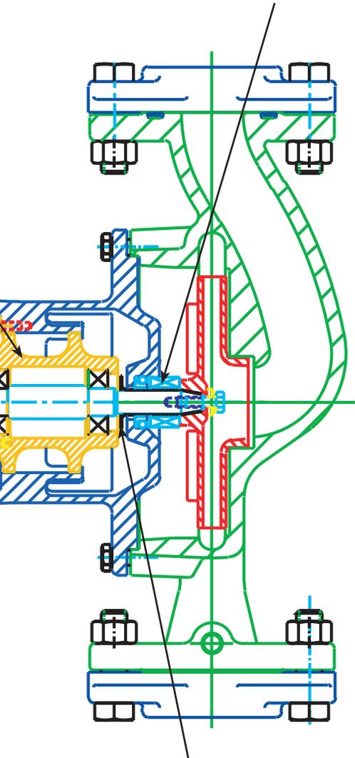
Replaceable corrosion resistant shaft sleeve incorporates a "built in" slinger to deflect water away from the bearing cartridge in the event of a seal leak.
